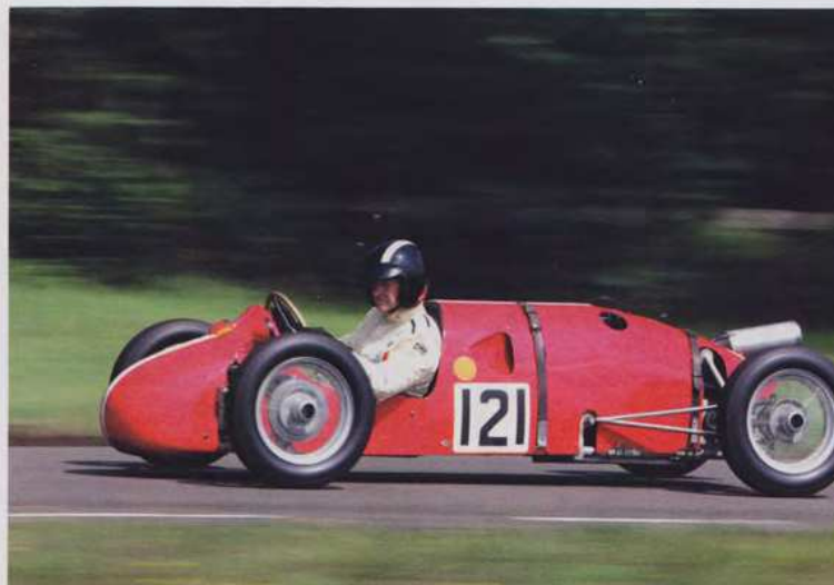
From top: Staride pushes driver to the front due to its enormous central tank; interweaved spring, brake, sprocket and fuel pump: a masterpiece of packaging
