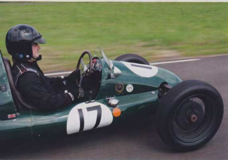
JAP-engined Cooper MkV has distinctive pannier tanks, fuel moves to above driver's legs on curved-tube MkVIII (below), which packs a Norton Manx unit
