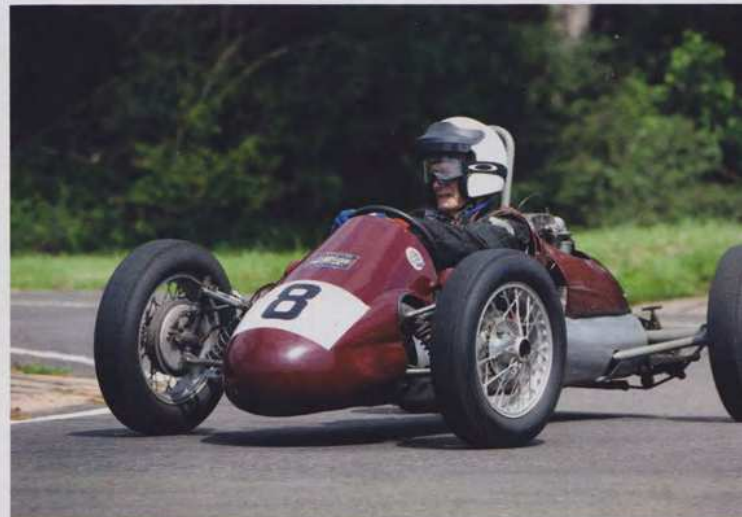
Martin pulls under-chassis transverse springs in tension (originally rubber bands) via chains and sprockets. Left: c50bhp double-knocker Norton
