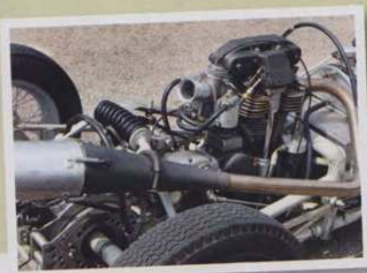
Martin pulls under-chassis transverse springs in tension (originally rubber bands) via chains and sprockets. Left: c50bhp double-knocker Norton
