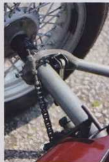
Martin pulls under-chassis transverse springs in tension (originally rubber bands) via chains and sprockets. Left: c50bhp double-knocker Norton
